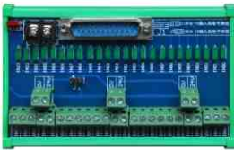
ADT-I24HNA Input splitter Size : 134 x 85mm
