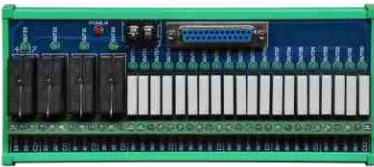
ADT-O24HNA Output splitter Size : 195 x 85mm
