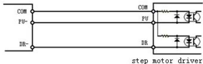
ADT-8830/8848 Single-Ended Wiring
